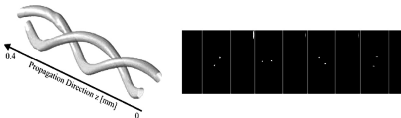
FIGURE 8 Nematicon interactions out of the plane ( y, z ). Left: sketch of spiraling Nematicons versus propagation. Right: images of the cluster in the output transverse plane ( x, y ) for various excitations: 2.1, 2.7, 3.3 and 3.9 mW in each beam, respectively. The boundaries of the NLC cell are indicated by vertical solid lines: as power increases, the cluster rotates faster, with a measured sensitivity of \pi/2 (rad)/mW.
